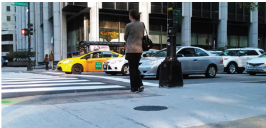
Figure 23 Small cell integrated into manhole cover. Source: Kathrein
